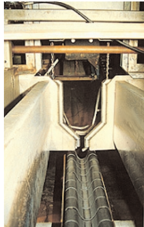
Figure 1: Headholder for double rail restrainer (left). This device holds the animal's head comfortably and allows a Rabbi to perform the Kosher cut with the animal quietly restrained. A cow's-eye view of the head holding device on the center track double rail restrainer (right).
