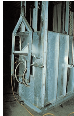
Figure 2: The ASPCA-pen is a well developed fixation device for ritual slaughter in an upright position (for more information see: www.grandin.com )
