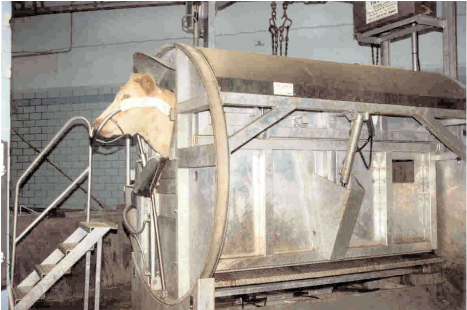
Fig. 1: Weinberg restraining device used for ritual slaughter and post cut stunning
